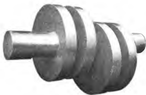
Fig. 2206. Built-up Disk Crank Axle.
